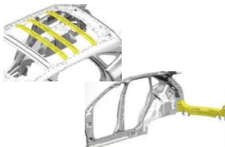
Steel-polymer composite Applications in BIW (Ford)
